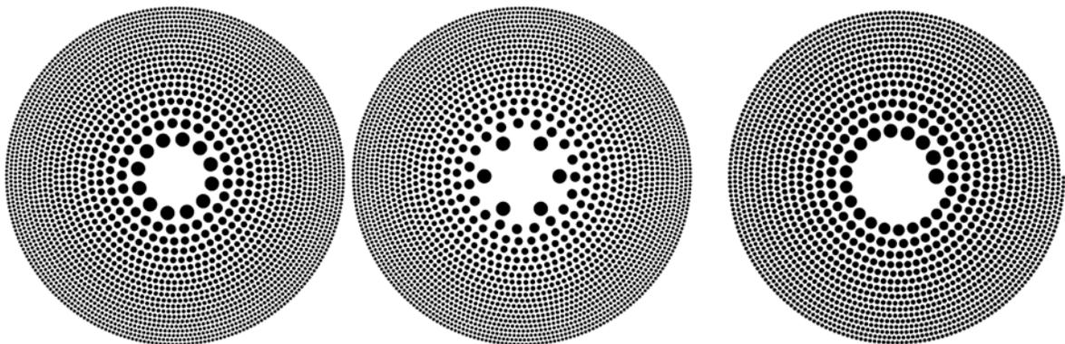
**Exhibit 7:** For intensity apodization, a standard photon sieve (left) can be modified to a Gaussian density profile (center) or spiral configuration (right) for different imaging properties.
