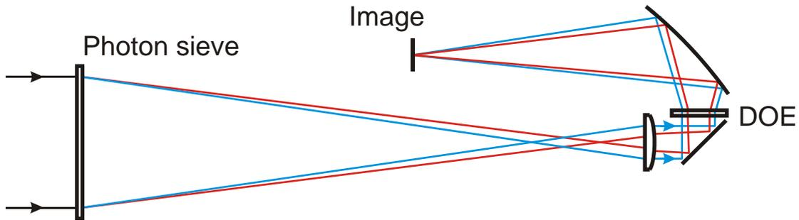
**Exhibit 6:** Broadband diffractive optic telescope concept using a secondary diffractive optic element (DOE) for chromatic aberration correction.
