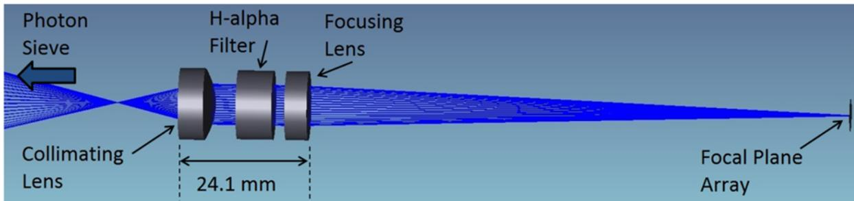
**Exhibit 3:** Peregrine telescope schematic. Focused light from the photon sieve (at left, not shown) passes through two lenses and filter. The collimated beam is approximately 10 mm in diameter, and the final focal distance from the second lens to the camera focal plane is about 100 mm. The three fold mirrors after the final lens are not shown.
