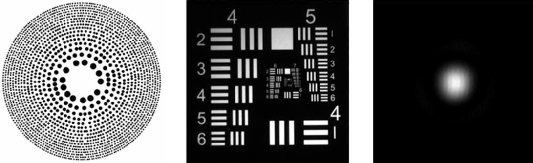
**Exhibit 2:** Magnified image of photon sieve (left) to produce diffracted images (center) and focal spots (right).
