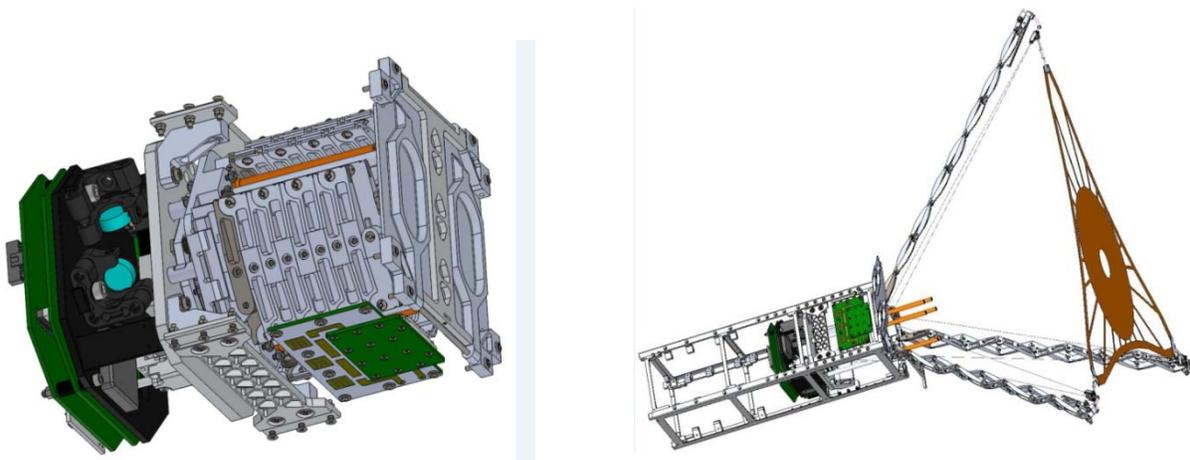
**Exhibit 1:** Stowed (1.5U) and deployed Peregrine payload schematics.
