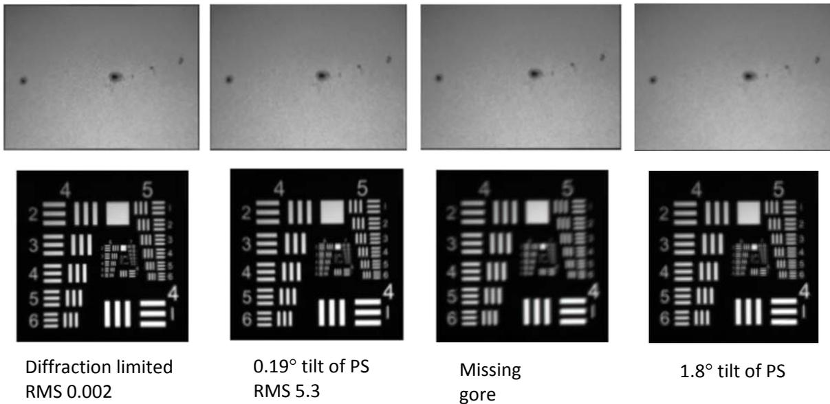
**Exhibit 4:** Simulated images of the Sun based on FS-7 expected performance: a) Diffraction limited performance; b) Based on deployment repeatability testing, 0.19° tilt in the primary optic; c) Based on worst-case-scenario deployment testing, tearing of a gore of the membrane is possible during deployment; d) 1.8° of tilt in the photon sieve is the maximum tilt error before clipping will occur.
