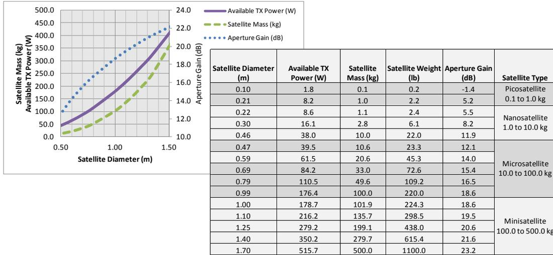
**Exhibit 6:** Spherical SmallSat Available TX Power, Aperture Gain and Mass
