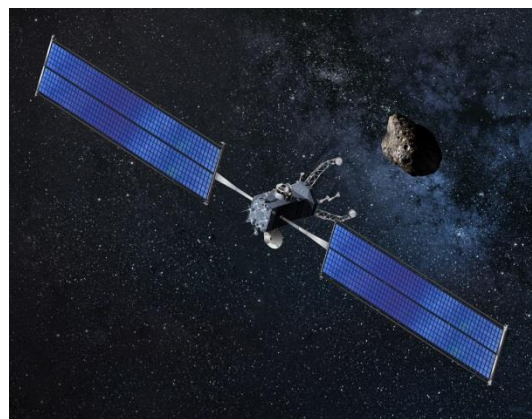
Figure 7. Block 0 50-kW Asteroid Redirect Vehicle with 3,600 kg Xe using current technologies
